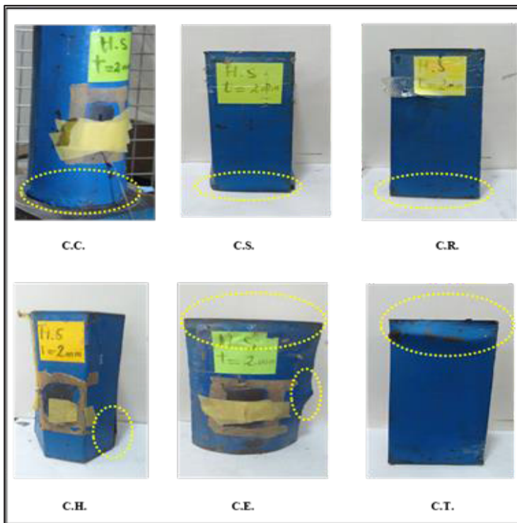
Figure 6: Failure patterns for all tested RACFST columns of steel tube thickness ( t ) = 2 mm.
