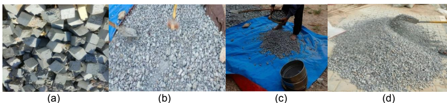
Figure 3: Details of recycled coarse aggregate: (a)The cubes and cylinders waste (b) Crushed concrete (c) Sieved the crushed concrete (d) mixes in proportions
