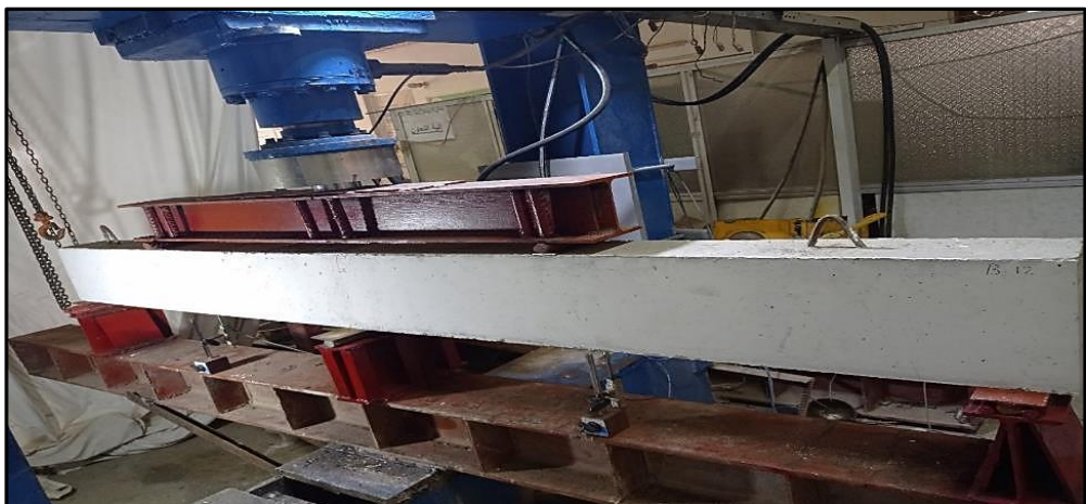
(b) Beam segment before applying the load.
