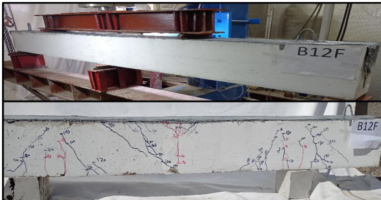
(e) Crack patterns in the tested extended continuous beams at the failure stage (BF12).
