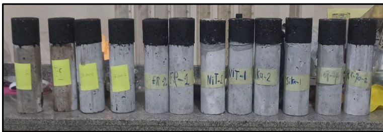
Figure 1: Composite Specimens used in a direct shear test.
