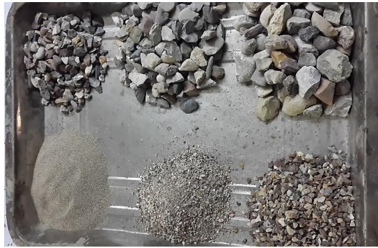
Figure 6: Selected surface course gradation to produce RAP mixtures.
