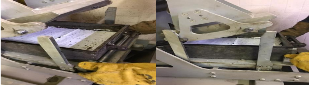
Figure 8: Shows how to compress the sample with the piston device.
