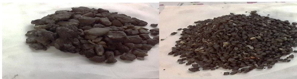
Figure 5: Fractionated samples (coarse and fine) of the reclaimed asphalt pavement (RAP).
