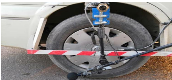
Figure 1: Sound intensity probe on the test vehicle.
