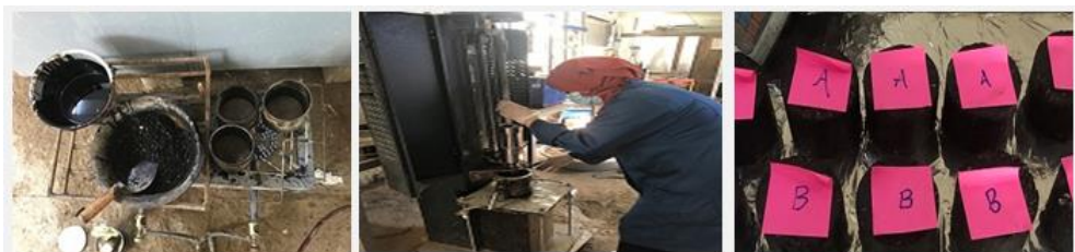
Figure 5: Prepare samples for Marshall Test.
