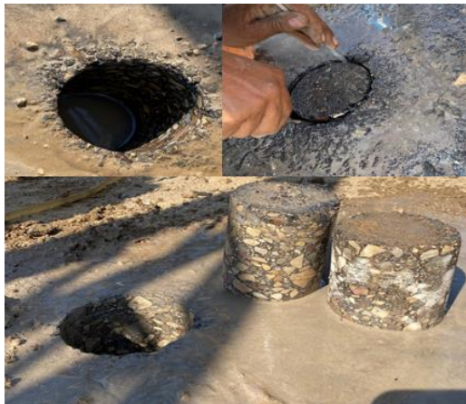
Figure 3: The extraction process.
