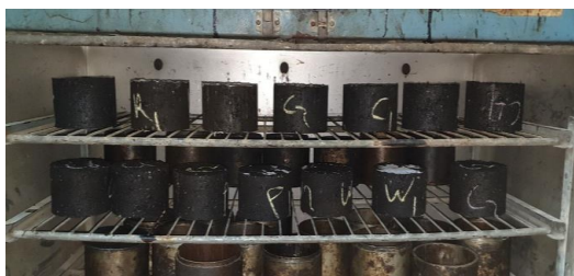
Figure 7: Sample in the oven at 85°C for 2 days.
