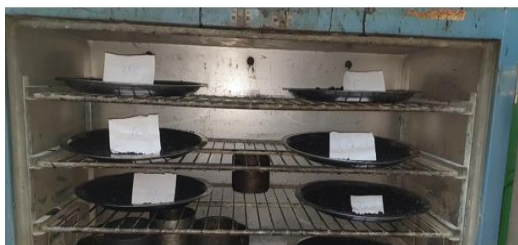
Figure 6: Sample in the oven at 135°C for 4hr before compaction.
