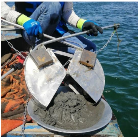
Figure 4: Van Veen Grab device.
