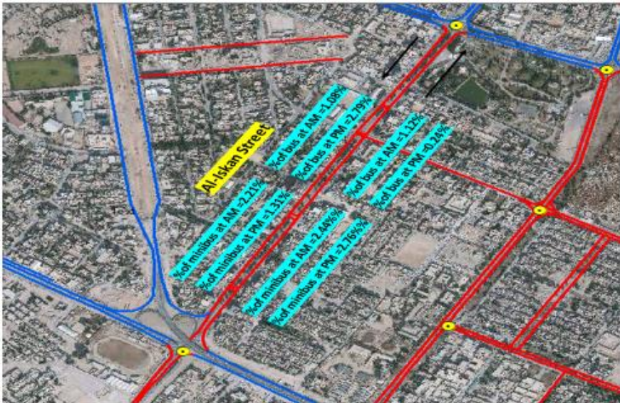
Figure 8: The average ratio of bus and minibus in GIS for Al-Iskan Street at AM and PM.
