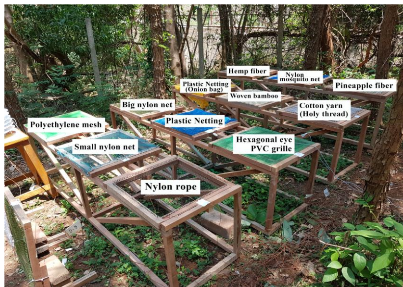
Fig. 5. Fiber installation in the test area
