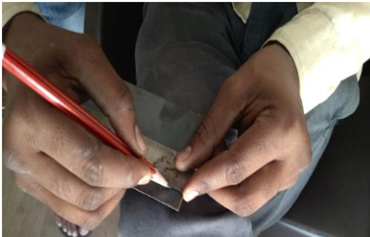
Fig.6. Marking dimensions (step -1)
