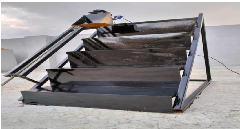
Fig.9. Finished prototype of a staircase lifter(step-4)
