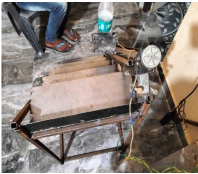
Fig.8. Assembling the mechanism to the staircase (step -3)
