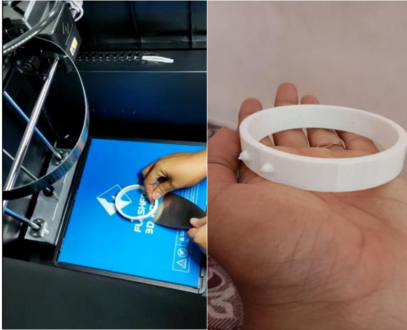
Fig. 1. (a) 3D Printing; (b) PLA Prototype.
