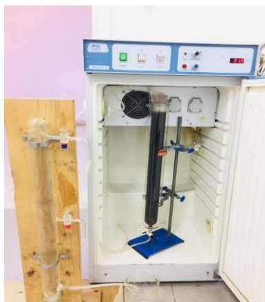
Fig. 1. A photograph of the column bioreactor connected to cylindrical glass collector
