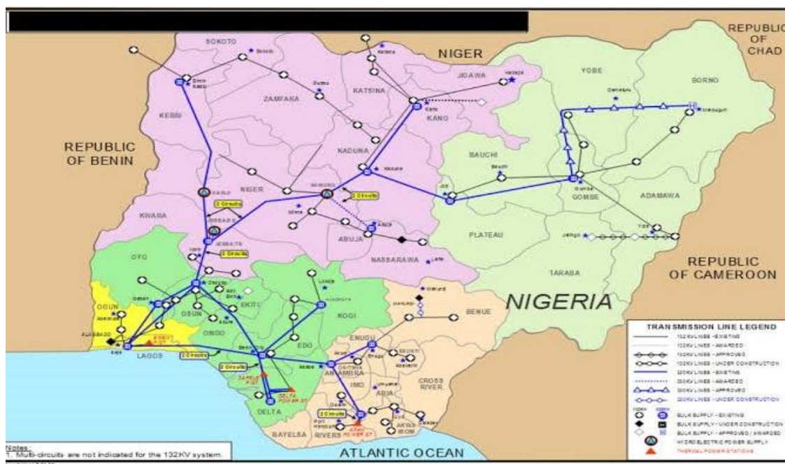
Fig. 1. existing TCN transmission line system
