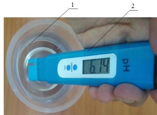
Fig. 11. The process of determining the pH of water. 1 – water; 2 – pH meter
