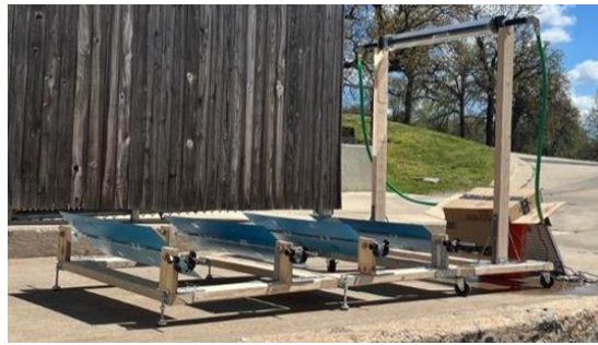
Fig. 9. Concentrator and receiver configuration for testing
