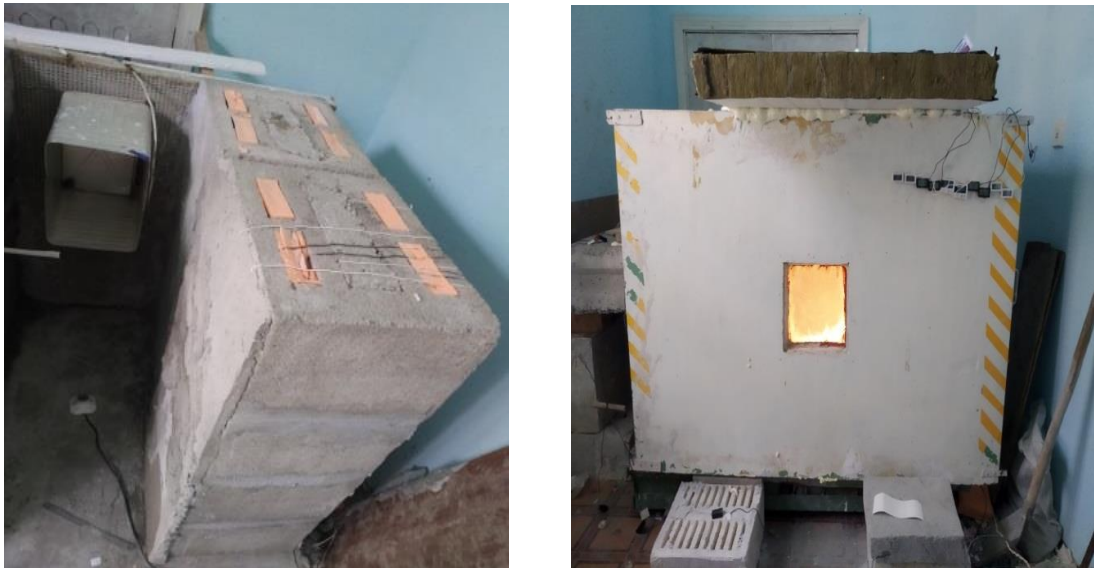
Fig. 1. Installation of thermosensors on the external wall sample of non-homogeneous gas block and general view of the climate chamber
