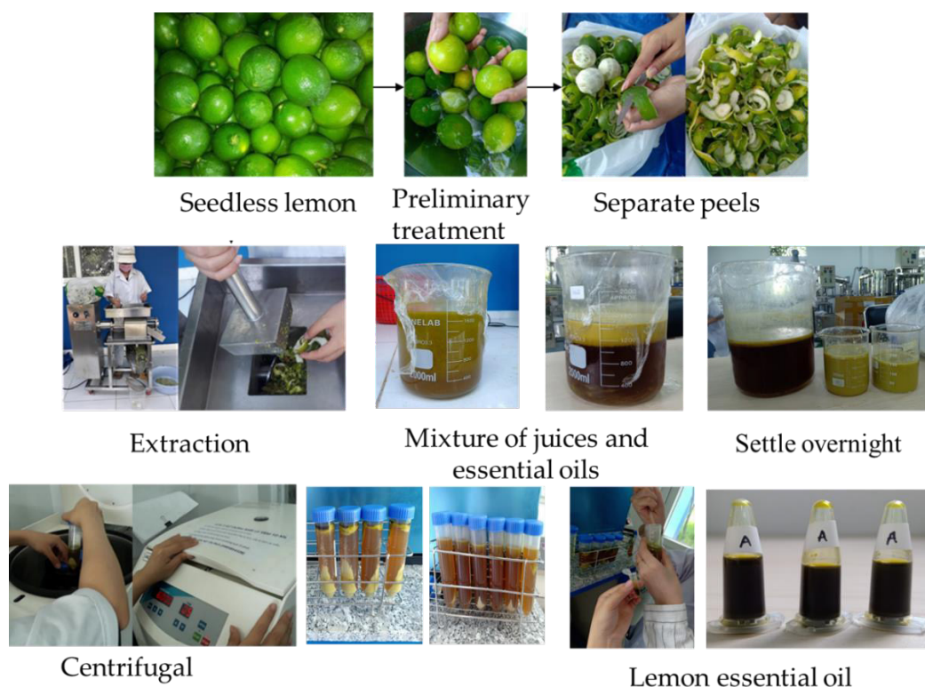
Fig. 1. Technological process of producing essential oils by pressing method
