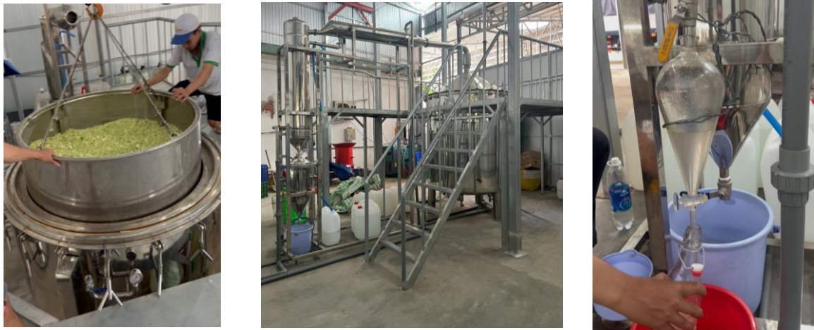
Fig. 1. Pomelo essential oil extraction system
