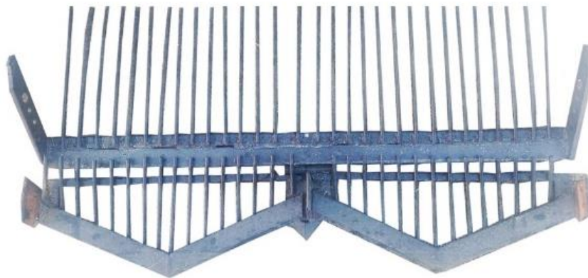
Fig. 2. Lattice ploughshare and honeycomb lattice ploughshare
