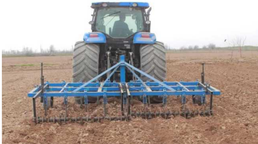
Fig. 2. A view of the working process of chisel-cultivator equipped with a rotary softener
