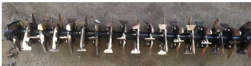
Fig. 1. Rotary softener equipped with shovel and straight flat blades.
