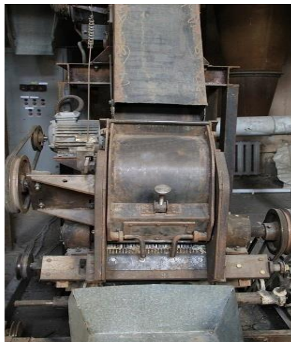
Fig. 5. Working chamber 30 saw linter 5LP
