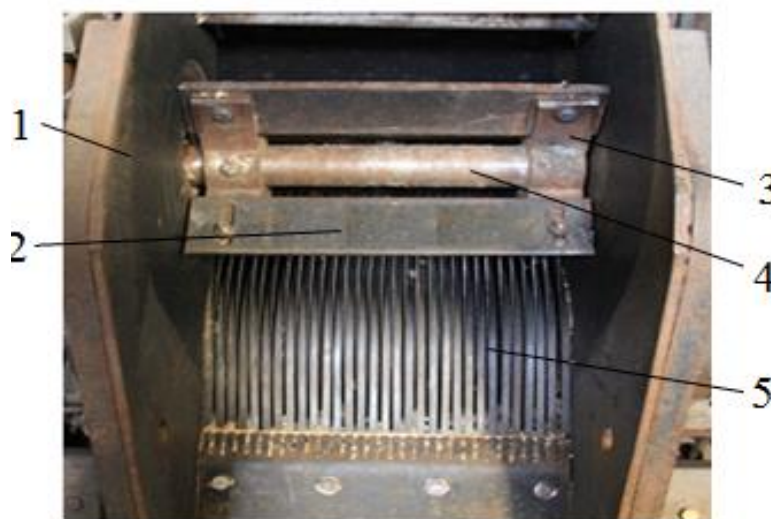
Fig. 6. Working chamber 30 of the saw linter with a serial turner: 1 - working chamber, 2 - blade, 3 - cross, 4 - shaft, 5 - saw cylinder
