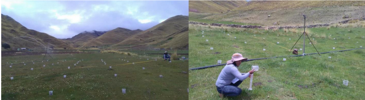
Fig. 1. Configuration and measurement of water heights in rain gauges
