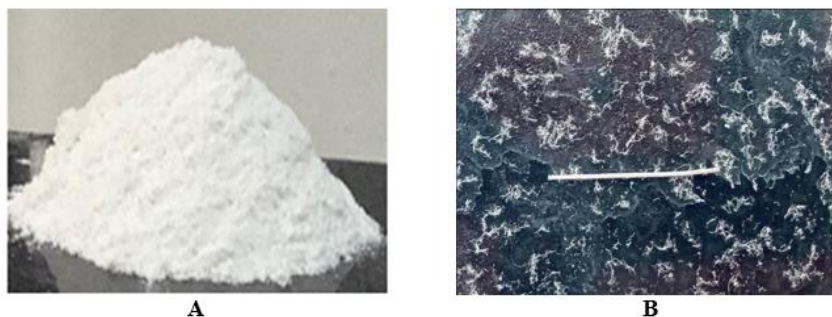
Fig. 1. A - Sample MCC; B – micrograph of milk thistle cellulose fibers (wire diameter 0.3 mm).
