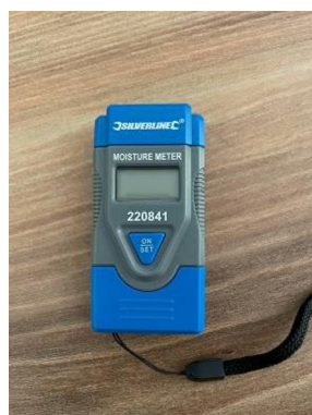
Fig. 10. Silverline Digital Moisture Meter. (Source: Authors).
