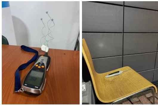
Fig. 5. A. Testo 435-2 during measurements; B. Outdoor Wi-Fi sensor. (Source: Authors).
