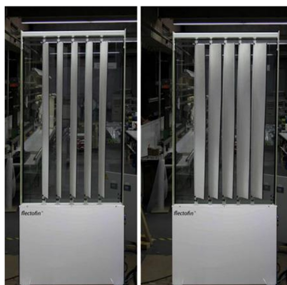
Fig. 15. Prototype of the Flectofin R shading system, in 1:1 scale, produced with industrial project partner Clauss Markisen (CM). Made of GFRP (height = 2 m, width = 0.25 m, and
