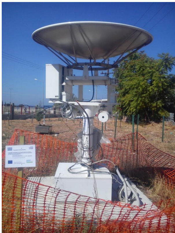
Fig. 1. The 2m S-band Dish at the premises of the Hellenic Open University Campus. The dish is currently under conversion to a radio telescope capable to monitor the 10.7cm solar flux.
