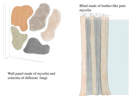
Figure 7. Concept design for possible application of fungi with sclerotia as wall panel and blind.
