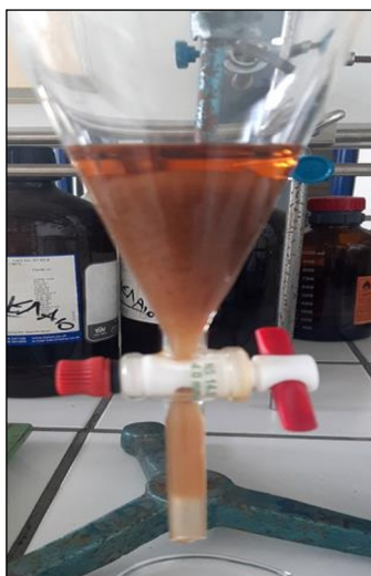
Fig. 1. Two-phase separation after the esterification process.
