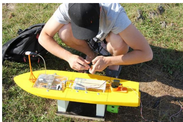
Fig. 1. Self-made boat model, equipped with propulsion and control equipment and data transmission.
