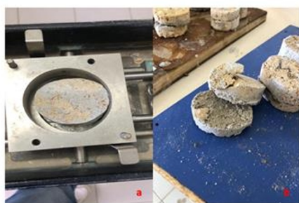
Fig. 4: (a) Closeup view of the shear test machine and tested samples (b)
