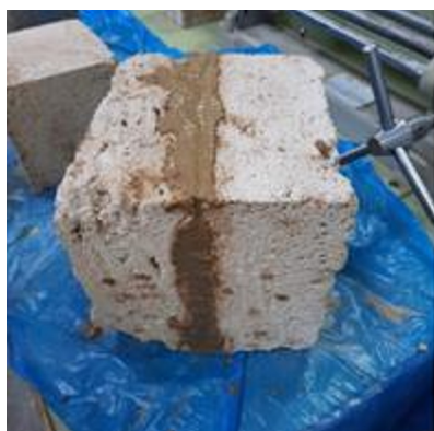
Fig 2. Geopolymer paste used on the sandstone rock.
