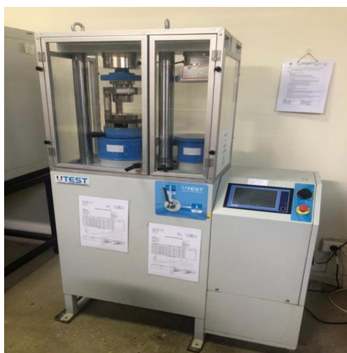
Fig. 1. UTCM-3744 used for compressive strength testing.
