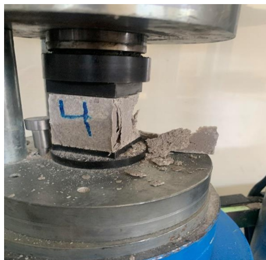
Fig. 2. Compressive Strength test conducted on a sample.
