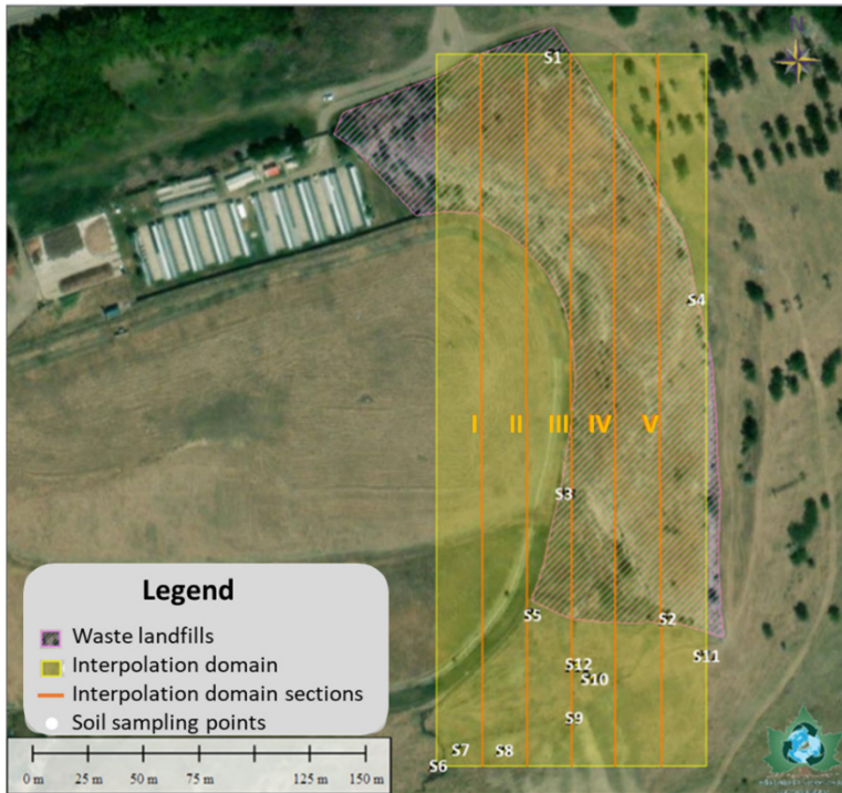
Fig. 2. Localization of the three-dimensional interpolation range of element values in soil samples
