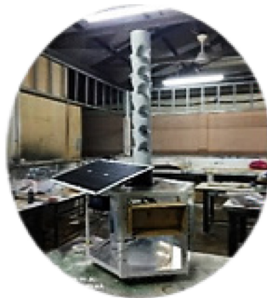
Fig. 5. A completed vertical hydroponic systems (VHS) embedded with Node MCU ESP32 and micro phyton and solar panel.
