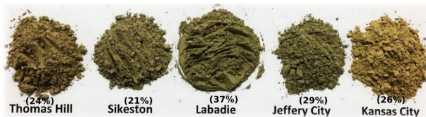
Fig. 6. Various colours of FA, which collected from different regions, based on CaO content (modified and redrawn from Gomaa et al. [84])
