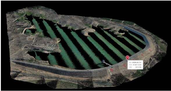
Fig.2 Digital point cloud 3D model of Lujiayao reservoir
