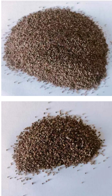
Figure 2-1: On-Site Collection of Backfill Sand Samples
