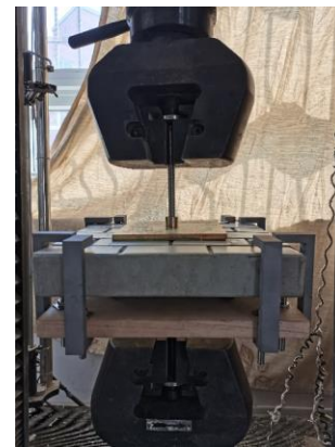
Figure 2. Setup for pull-off test.
