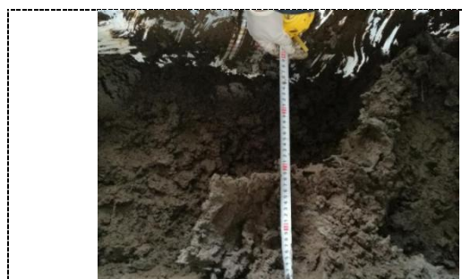
Figure 7. Expansion of grouting liquid in dense soil
