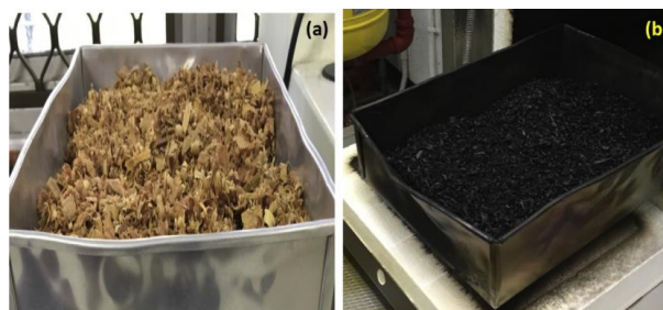
Figure 3. (a) Wood saw powder used in the preparation of biochar; (b) Preparation results of biochar. [26]
