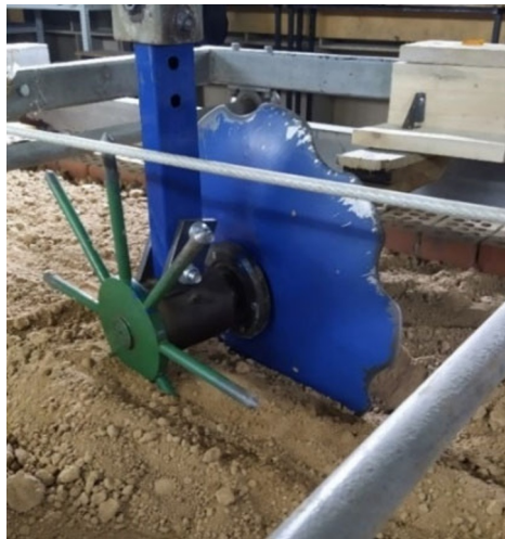
Fig. 5. A prototype of a disc-pin working body.
