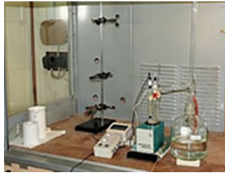
Fig. 2. Determination of oil alkalinity in laboratory conditions.
