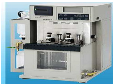
Fig. 1. The process of determining the viscosity of engine oil at temperatures of 40 and 100 °C.
