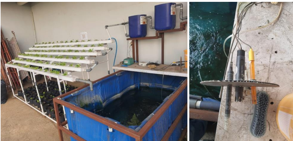
Fig. 6. Some sensors implemented in an aquaponics system
