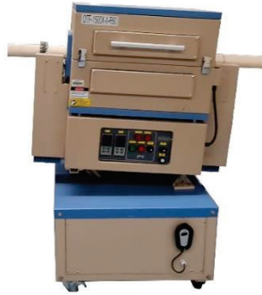
Fig. 3. Double heat zone rotary furnace used for sintering.
