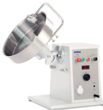
Fig. 2. Pelletizer used to convert W-CCA paste into green pellet.
