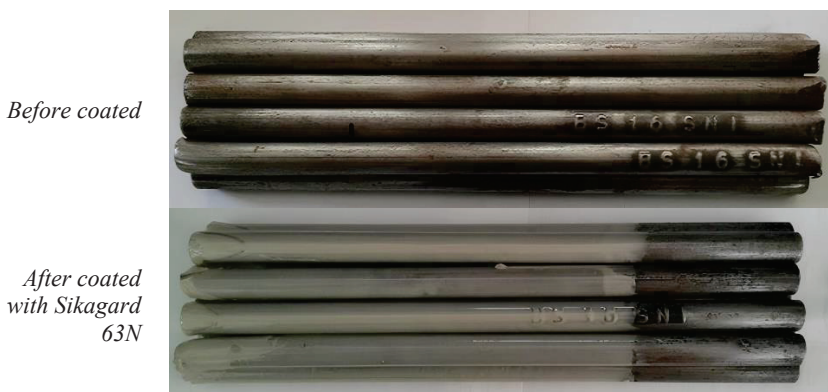
Fig. 2. Steel reinforcement coating.
