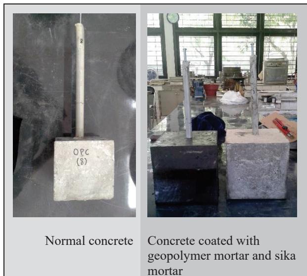
Fig. 4. Cube specimen before and after geopolymer mortar coating.
