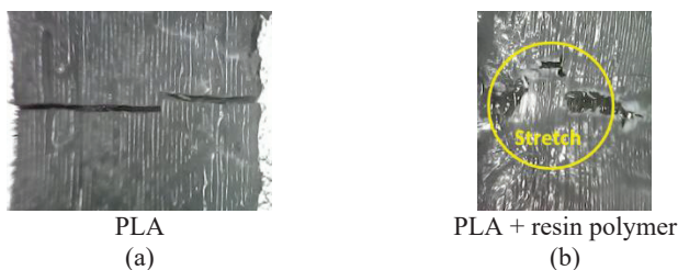
Fig. 4. Fracture characteristic a) brittle fracture and b) ductile fracture.
